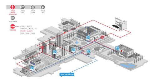
LEWsystem Apator prepayment system— comprehensive solution enabling the sale of electricity in prepayment system where it is purchased by individual consumer of specified volume of kWh • **Metering data analysis** - IT systems supporting the management of metering information
