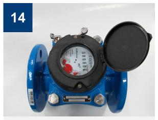
The MWN50-NKP water meter (NK transmitter installation ready); IP68-rated rotating counter features a single-magnet fixture installed at the x 0.01 position -> pulse rate at 100 L = 1 pulse.
