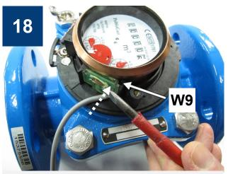
Press in the other end of the transmitter in the direction shown with the arrowhead pointing to the driver bit, into the other guide slot (see view W9).
