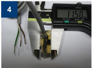
NO transmitter, P/N **31-7112-010000**, width b = 11.5 mm for IP65-rated water meters. Specification: Us = -5 to 24VDC; NPN OC; Is <30 mA (I =0 mA); YTLY cable 3 x 0.25 mm2 L = 2 m
