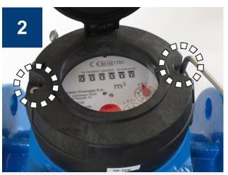
Remove the two Allen bolts and remove the counter guard assy.
