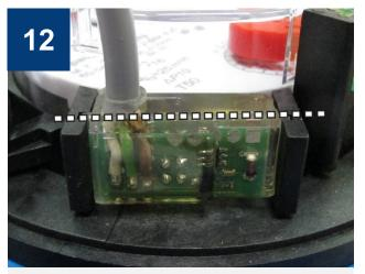
Complete the NO transmitter installation by engaging the NO transmitter into the guide piece to stop. The top of the NK transmitter should now be level with the top of the guide piece.
