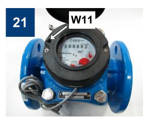
Install the counter guard assembly on the counter mechanism with the transmitter installed so the transmitter cable goes out of the counter guard via the respective cable entry at the "100 L = 1 pulse" label. Secure the counter guard with the two Allen bolts. Install the Allen bolt for the lead tamper seal wire in the hole next to the guard cover lug W7 in the counter guard to facilitate sealing of the water meter.
