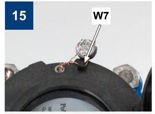
Cut the wire and remove the lead tamper seal with the Powogaz mark "KJ3". Remove the two Allen bolts which secure the counter guard. Remove the counter guard; note that the bolt at the guard cover lug W7 has the cap head designed to accommodate a lead tamper seal wire.
