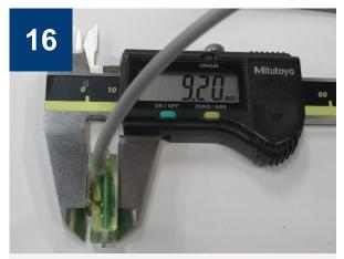
Install the NK reed relay pulse transmitter, P/N **31-8027-010000**, width b = 9.2 mm, intended for water meters and flow transducers (T50 and IP68). Specification: U < 24V; Is < (max 100 mA); cable: YTLY 2x0.14 mm<sup>2</sup>, L = 2 m.
