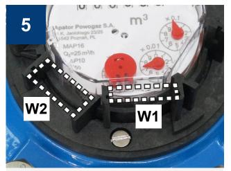
View of the counter mechanism installed in the retaining ring, with the counter guard removed. View W1: the installation location of the NK transmitter assembly. The magnet fixture is installed at the x 0.001 (DN40) indicator to enable a pulse rate of 10 L = 1 pulse.
