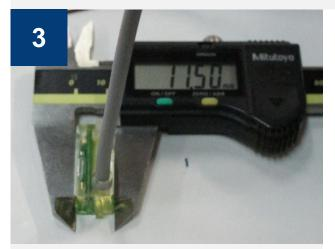
NK transmitters, P/N **31-8027-010000**, width b = 11.5 mm for IP65-rated water meters. Specification: U < 30VDC; Is < (max 100 mA); cable: YTLY 2x0.14 mm<sup>2</sup>, L = 2 m
